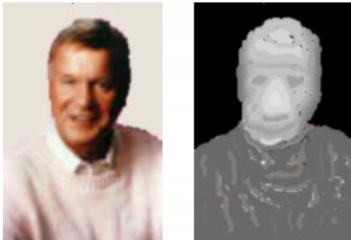
Figure 1. An intensity image and grayscale-coded depth image of a person. Since the background is similar color to the person's shirt, it is difficult for the computer to segment the person from the background using the intensity image. The segmentation is trivial using the depth image.
